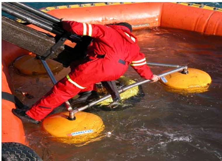
Figure 18: The use of mechanical skimmers for spilled oil recovery (Source: Markleen, 2020)
