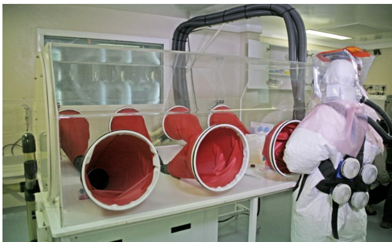
Fig.7. The Present CIRMF High Security P4 Laboratory with “Glove Box”.
