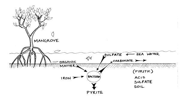
Figure 2: Biogenesis of pyrite formation in coastal mangrove soils (Smith et al., 1995)
