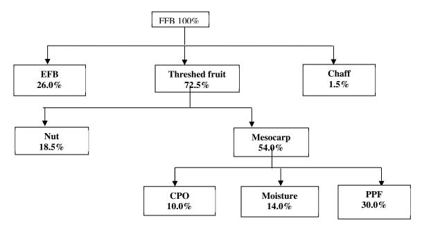
Figure 16: Material mass balance of semi-mechanized oil palm processing in Bayelsa state
