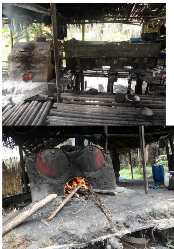
Fig. 28: Rudimentary ethanol distillation equipment used in the Niger Delta
