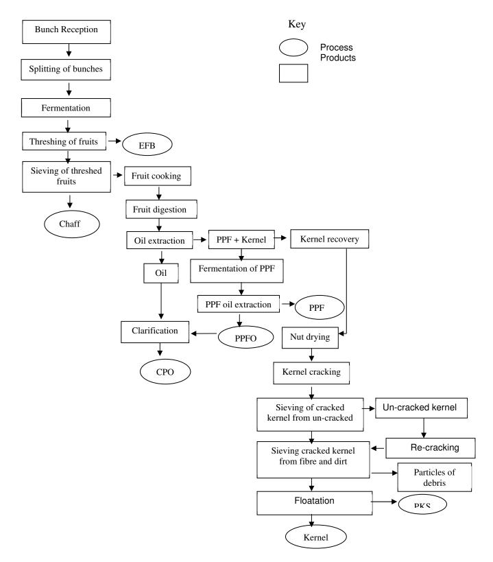
Fig. 14: A flow chart of small holder oil palm processing in the Niger Delta (EFB = empty fruit bunch; PPF = palm press fibre; CPO = crude palm oil; PPFO = palm press fibre oil; palm kernel shell)
