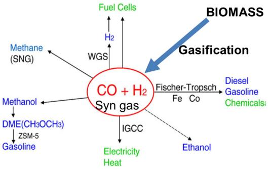
Fig 8: Commercially available fuel products from syngas produced through biomass gasification (modified from Zhang, 2010). WGS= water gas shift; IGCC= integrated gasification combined cycle
