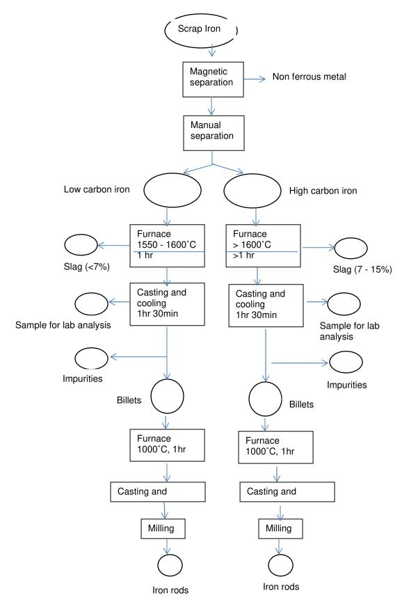
Fig. 26: Scrap iron and steel recycling in Nigeria (Ohimain and Jenakumo 2013)
