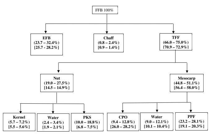
Fig. 15: Material-mass balance of FFB processed by small holders in Nigeria (**Ohimain** et al 2013f). Figures in bracket are the percentage of the different fraction of FFB: () = Dura variety; [] = Tenera variety.
