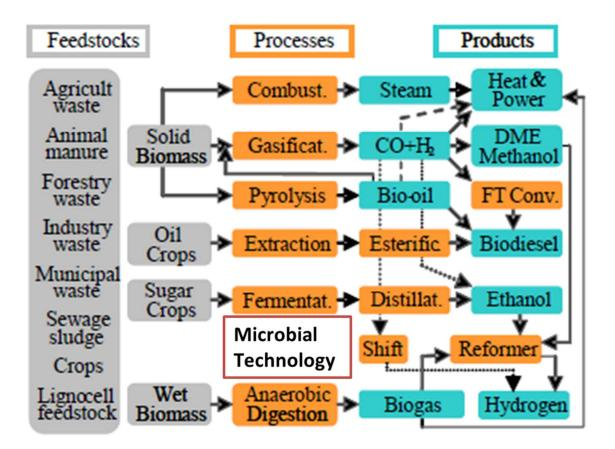
Fig. 7. processes for the conversion of waste biomass to various energy carriers Source: Modified from **OECD/IEA 2007**
