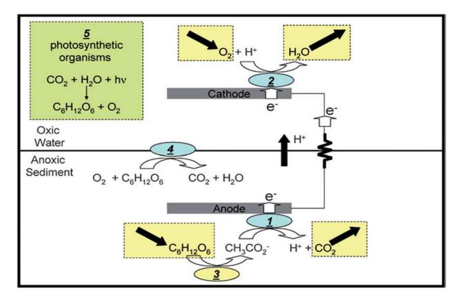
Fig 11. Schematic depiction of simplified mechanism of power generation by the benthic microbial fuel cell (BMFC): (1) biofilm catalyzed anode reaction; (2) biofilm catalyzed cathode reaction; (3) fermentative reaction, (4) the microbial oxygen barrier and (5) photosynthesis for the microbial photo-electrochemical solar microbial fuel cell (SMFC). (Source U.S. Naval Research Laboratory)
