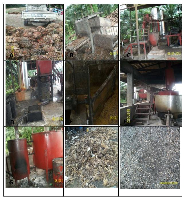
Plate 25: Semi-mechanized oil palm processing; [A] FFB reception [B] Stripper, [C] sterilization/boiling, [D] Digestion and oil extraction zone [E] Clarification zone [F] dryer, [G] Storage of CPO
