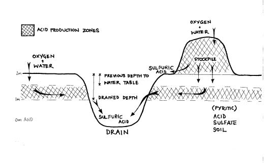
Fig 3: Microbial oxidation of pyrite causing the release of sulphuric acid (Smith et al., 1995)
