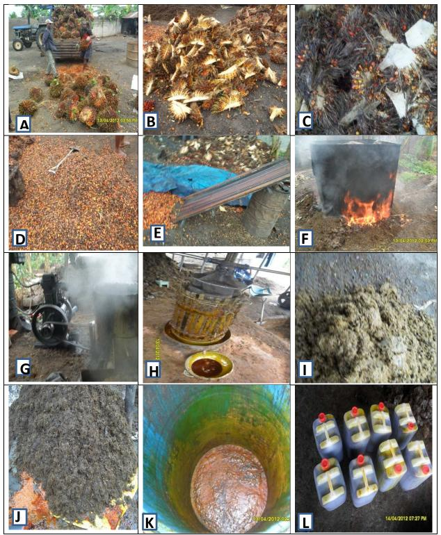
Plate 24: Pictorial show of oil palm processing by smallholders in Nigeria; [A] FFB reception, [B] Slicing of FFB, [C] Fermentation of sliced fruit, [D] Threshed fruit, [E] Sieving of threshed PF, [F] Boiling of PF in a barrel, [G] Digestion of boiled PF, [H] Oil extraction, [I] Fiber and nut [J]Fermentation of PPF, [K] Clarification drum [L] Storage of CPO
